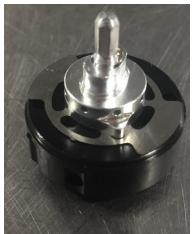
4. If the fork has a 3-position mode selector switch, use the blue knob to turn it to the middle of the 3 clicks. This ensures that the two pins poking through the butterfly valve align with the correct C-shaped slots in the piston (the pins are not the same size, nor are the slots).
