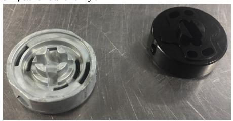
3. Reinstall the mode selector switch and butterfly shim into the topcap assembly as per factory service manual. Check the orientation carefully! It is easy to put the butterfly shim onto the mode selector upside down - it will not work like this.
