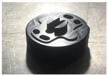
6. Install shim stack onto the shim tabs on the Fractive piston - largest shim first - while the topcap/Fractive piston are upside down. Ensure shims are correctly oriented - largest diameter shim should be against the piston, smallest diameter shim should be at the back of the stack, furthest from the face of the piston. Picture below shows piston with and without shims. They are on the opposite side of the piston to where the butterfly valve and mode selector engage.
