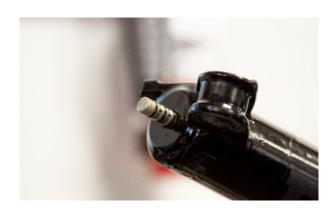
**1.10** Place installation tool over footstud & wind down nut. Use an 11mm socket to pull the shaft through until you feel minor resistance. Don't do it up tight. Remove installation tool.
