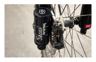
**2.10 Using the torque wrench,** torque to 50in/lbs (5.6Nm) whilst holding the Secus in place. You can loosen the footnut at any time to relocate it - the rotational position does not matter for function, only for clearance and minimising protrusion of the Secus.
