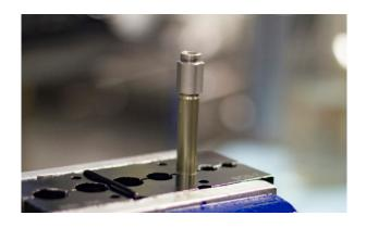
**1.3** Heat area with heat gun.Remove foot stud from shaft using 14mm wrench or knipex, do not use multigrips.
