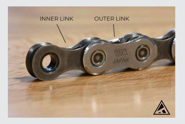
An S4 Supernought, for example, will require five inner plates and five outer plates, a total of 10 links, to be removed to shorten the chain from 126 to 116-links total. For chains that utilize a 'quick link' to connect the chain, the quick link itself will count as one of the outer plates. A quick way to count the links in your chain is to count all of the outer links, including the 'quick link' and double it. For example a 126 link chain will have 63 outer links (including the quick link).
