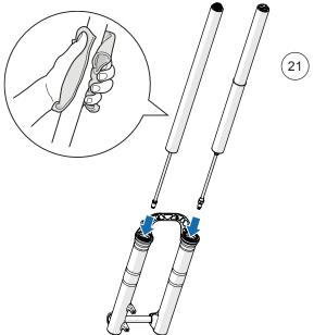
22. Inject 10 ml fork lubrication on both sides.
