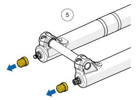
**6.** Use a 14 mm wrench to hold the rebound adjuster knob steady. With a 2 mm hex wrench remove the screw and the knob.
