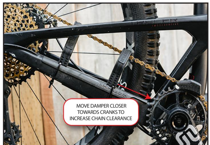
9. Once you are happy with the position of your STFU damper, add the additional cable tie to properly secure the unit to your frame. We like to position the cable tie heads on the underside or even back side of the chainstay so they are not seen. We recommend using a pair of pliers to really tighten the cable ties up so the dampers are as secure as possible.
