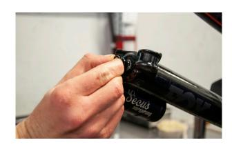
2.3 Use a torque wrench to torque the footnut to 50in.lbs (5.6Nm) in order to fully seat the assembly. Do not exceed 50in.lbs or you will break things. DO NOT tighten without a torque wrench or you will break things.
