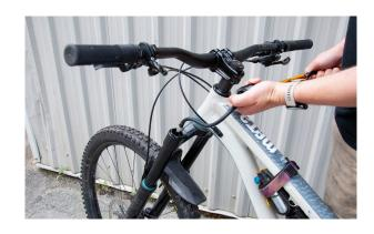
**3.2** Push down slowly onto fork to equalize (this will be difficult - you can do it at a lower pressure initially). You will hear a hissing sound as the air from the positive chamber passes through the ports into the negative chamber. As this occurs, the pressure in the positive chamber will drop.
