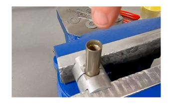
**1.5** Place a drop of red Loctite onto Secus footstud thread. Do not get any on the o-ring.
