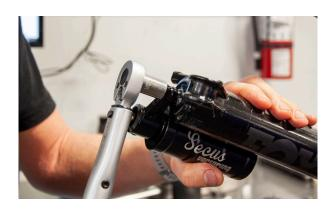
2.4 Install the fork back onto your bike at this stage. Also install your front wheel & ensure brake caliper is aligned as per normal.
