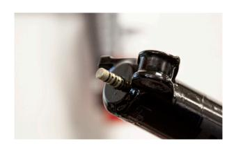
**1.9** Place installation tool over footstud & wind down nut. Use an 11mm socket to pull the shaft through until you feel minor resistance. Don't do it up tight. Remove installation tool.
