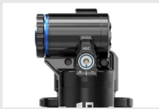
For the **Supernought** we recommend 28 - 30% sag (or 21 - 22.5mm of shaft insertion). **Please reference the chart on page 02 for your recommended spring weight.** These spring weights will provide approximately 30% sag.
