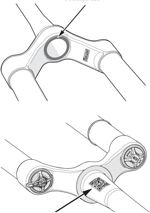
The part no of the fork can also be found on the steerer tube as a QR-code. Use a QR-code reader in a smartphone to receive the part no.
